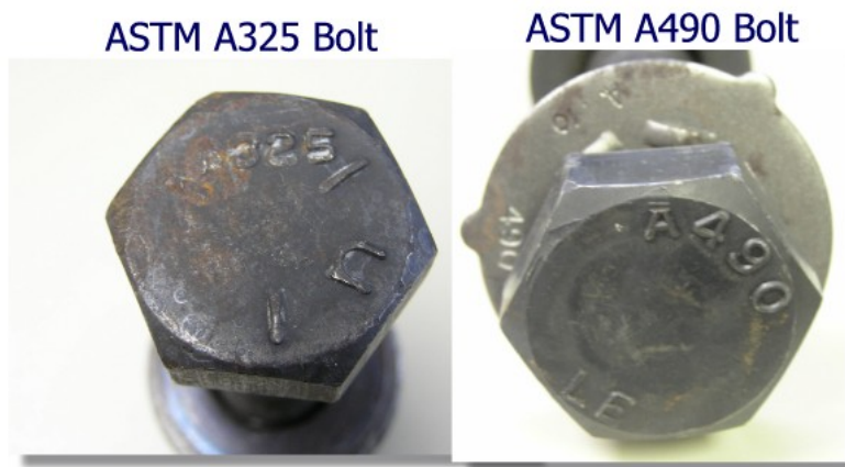
Figure 2.3.2 Bolt Identifiers
