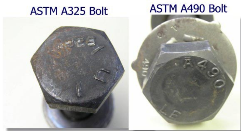
Figure 2.3.2 Bolt Identifiers
